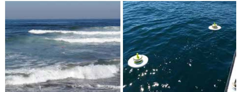
Figure 16: Lagrangian drifters, March 2018 field campaign in Cartagena Bay.
