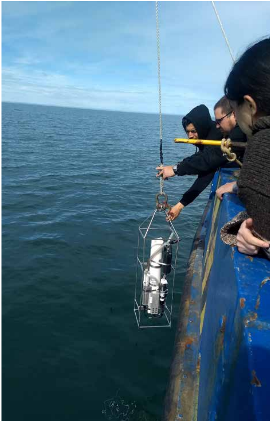
Figure 18: Deployment of a CTD during October 2018 Magallanes field campaign
