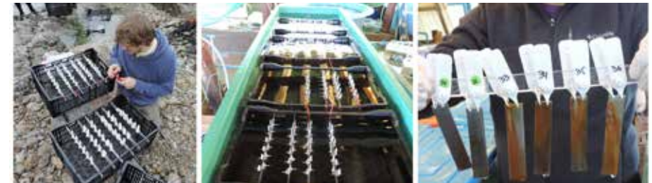
Figure 2: Exposure experiments of stainless steel coupons to seawater. Different types of tanks and configurations are used to simulate the effect of tides and immersion in the corrosion resistance of the tested materials.
