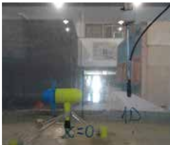
Figure 4: Acoustic measurements performed at the laboratory flume at DIHA-PUC, using an AS1 hydrophone, with a scaled Sabella turbine.
