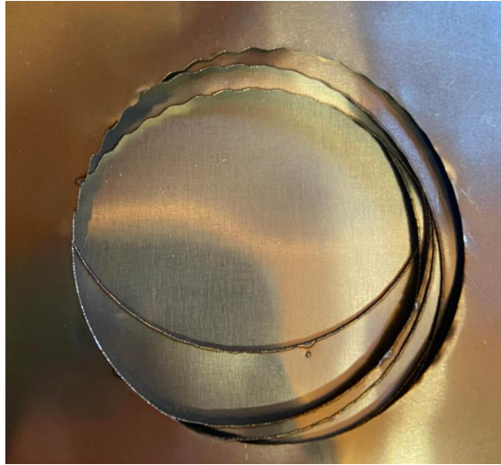
Figure 12. The cut head mount wasn't stiff enough to prevent oscillations during accelerations required for circle cuts, resulting in a wavy cut.
