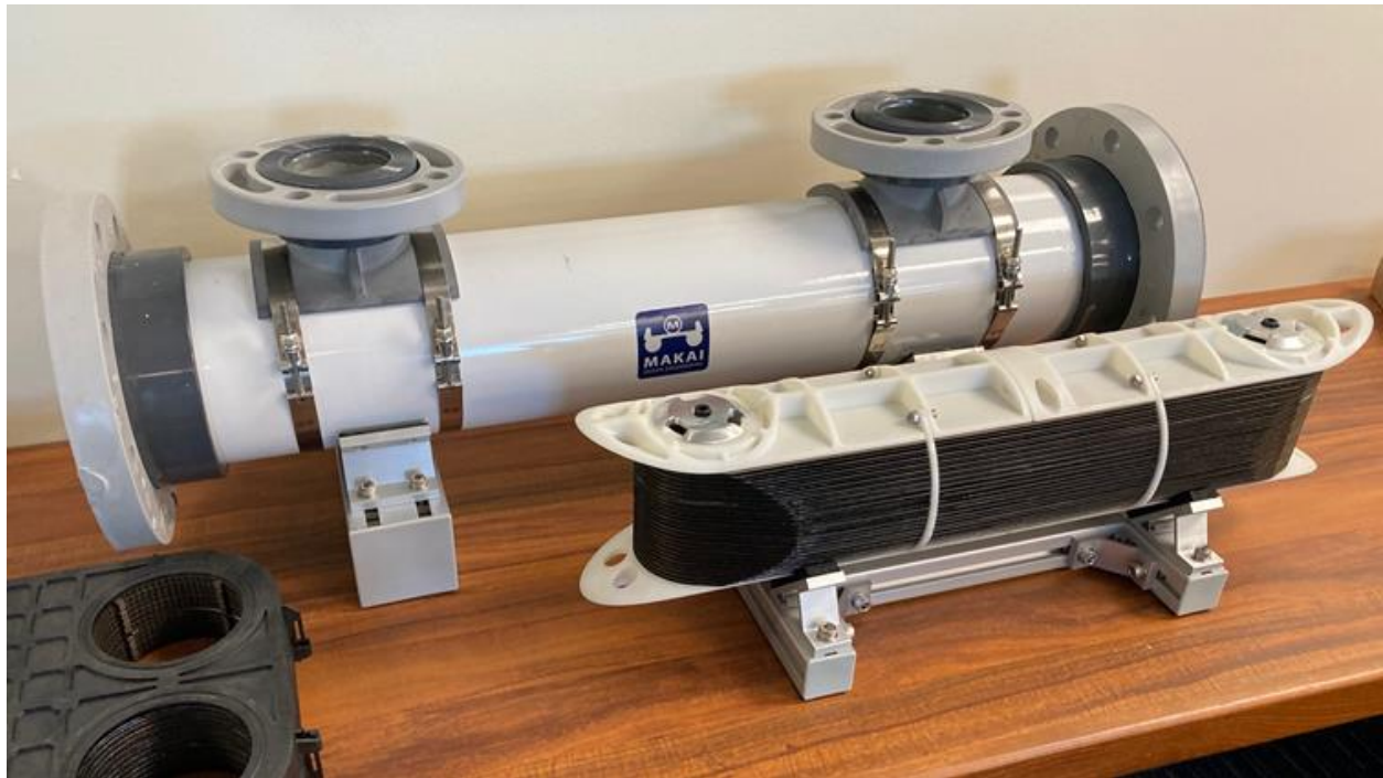
Figure 1. 6" TFPX prototype showing the housing and the plate stack.
