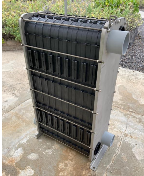
Figure 4. Demonstration of 9 modules stacked to form one full-length 4-port TFHX unit.
