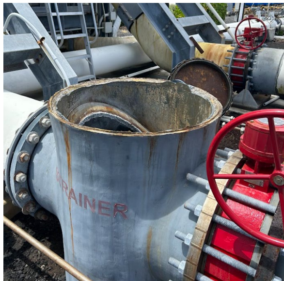
Figure 14. Top part of the strainer sheared off.
