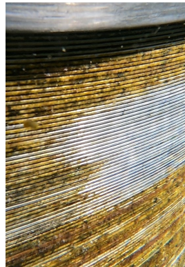
Figure 28. (top) Intake screen upon installation. (bottom) Intake screen after one year.
