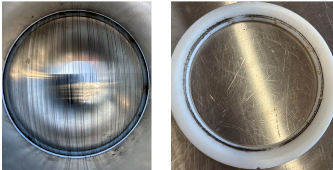
Figure 11. Weld slag in valve seating surfaces prevent quick-close valve from sealing.
