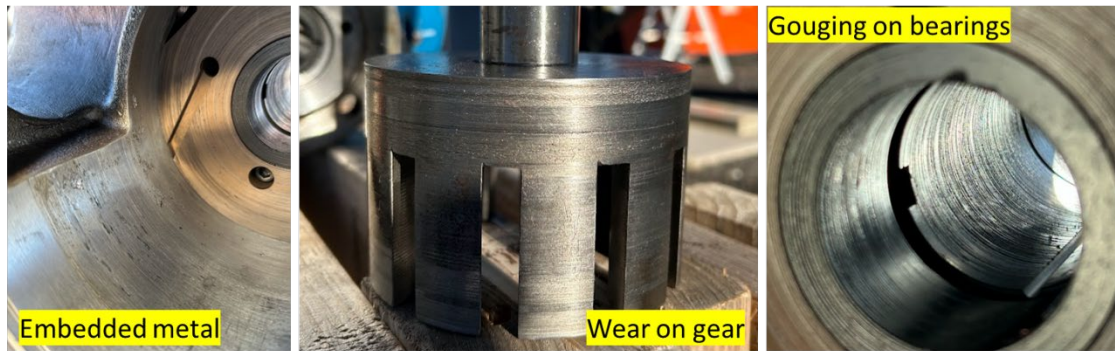
Figure 7. Recirc pump damage.
