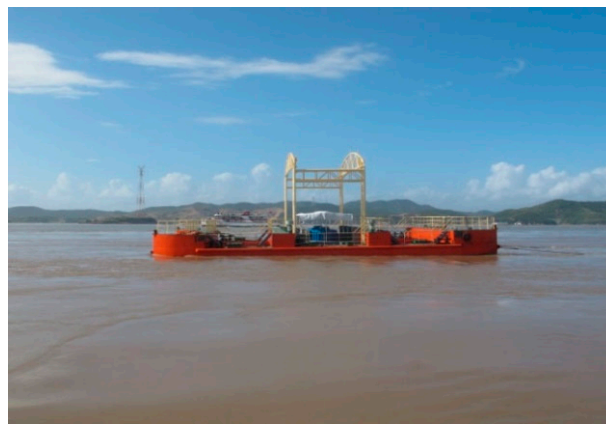
Figure 1. 2 \times 150 kW floating vertical current turbine system.
