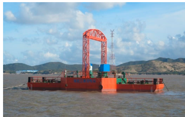
Figure 2. 2 \times 300 kW floating vertical current turbine system.
