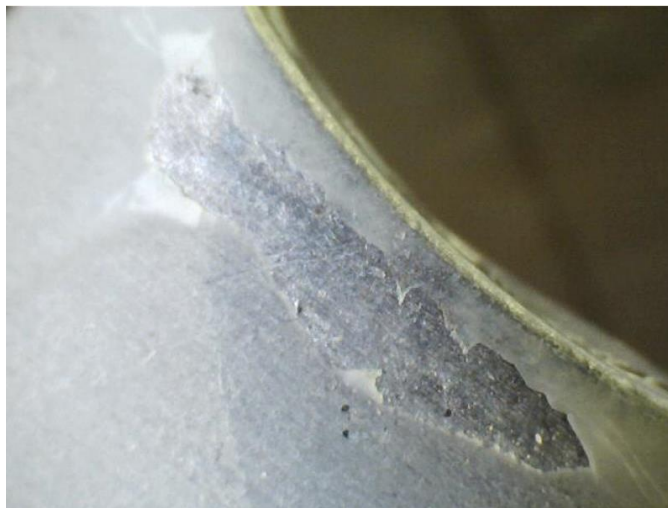
Figure 4-19. Typical SiloXel coating defect on in-line plate. Samples were still tested.
