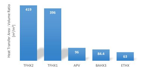
Figure 12. Comparison of heat transfer area to volume ratio for tested heat exchangers.
