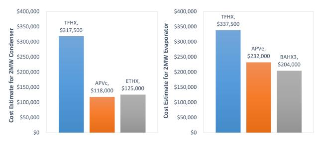
Figure 14. Comparison of estimated cost for 2MW heat exchanger.
