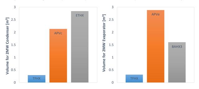
Figure 13. Comparison of required volume for 2 MW heat exchanger
