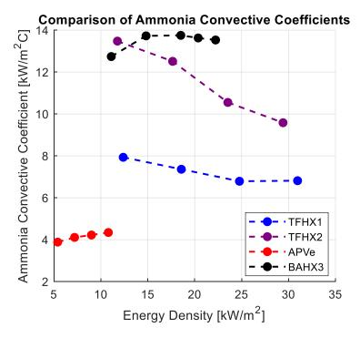
Figure 9. TFHX ammonia convective coefficients are ~2-3X higher than APV and ~0.5-0.85X lower than BAHX3 at the same energy density.
