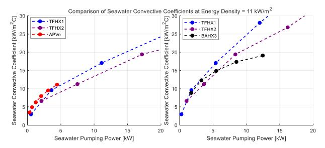
Figure 8. TFHX seawater convective coefficients are up to ~ 0.9X lower than APVe and comparable to BAHX3. Convective coefficients are plotted versus seawater pumping power to produce 3 MW for the APV comparison and 1.5 MW for the BAHX3 comparison at an energy density of 11 kW/m<sup>2</sup>.
