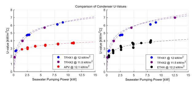
Figure 4. U-value vs Seawater Pumping Power comparison. TFHX's U-value is ~ 1.5X that of APVc or ETHX for the same seawater pumping power (through the heat exchanger only). Comparison with APV is scaled to 2.5 MW and comparison with ETHX is scaled to 2 MW.
