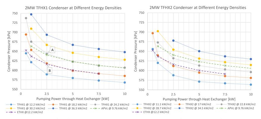
Figure 10. Comparison of condenser operating pressure versus seawater pumping power for 2MW TFHX condensers at various energy densities and 2MW APV and ETHX condensers. For the same seawater pumping power (through the heat exchanger only), the TFHX is capable of lower operating pressures at power densities up to 24 kW/m<sup>2</sup> compared to APVc (Point A) and power densities up to 18 kW/m<sup>2</sup> compared to ETHX (Point B).
