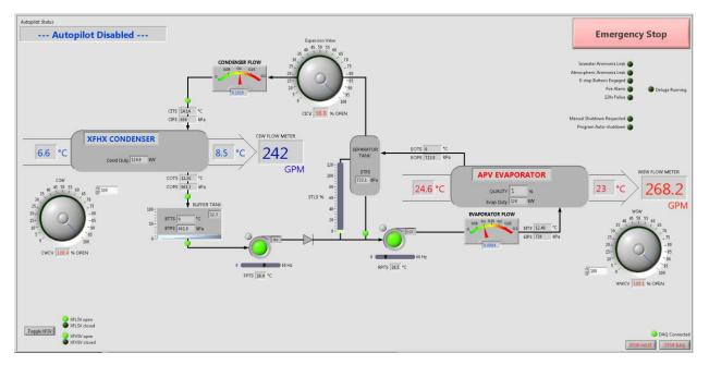
Figure 3. System overview page of the 100 kW Control Program. Seawater valves, the expansion valve, and feed and recirculation pumps can be controlled manually, locally, or autonomously.
