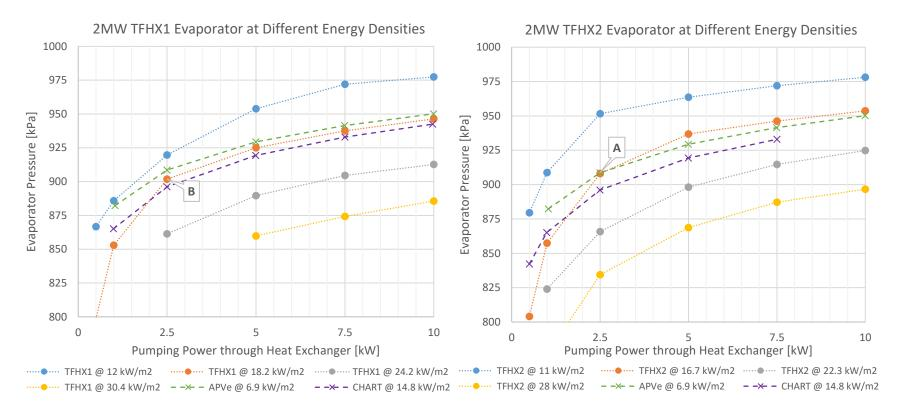
Figure 11. Comparison of evaporator operating pressure versus seawater pumping power for 2MW TFHX evaporators at various energy densities and 2MW APV and CHART evaporators. For the same seawater pumping power (through the heat exchanger only), the TFHX is capable of higher operating pressures at power densities up to 16 kW/m<sup>2</sup> compared to APVe (Point A) and at power densities up to 18 kW/m<sup>2</sup> compared to CHART (Point B).
