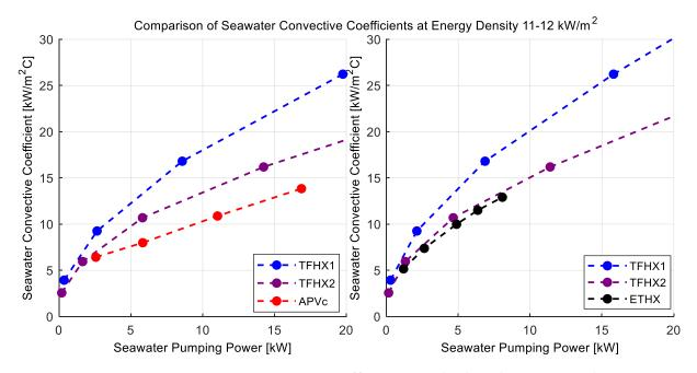
Figure 5. TFHX seawater convective coefficients are higher than APV and ETHX. Convective coefficients are plotted versus seawater pumping power to produce 2.5 MW for the APV comparison and 2 MW for the ETHX comparison at an energy density of 11-12 kW/m<sup>2</sup>.
