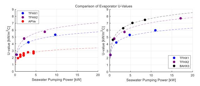
Figure 7. U-value vs Seawater Pumping Power comparison. TFHX U-value is ~ 1.2-2X that of APVe and ~0.7-0.9X that of BAHX3 for the same seawater pumping power (through the heat exchanger only).
