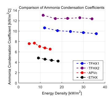
Figure 6. TFHX ammonia condensation coefficients are 1.5-3X higher than APV and ETHX at the same energy density.
