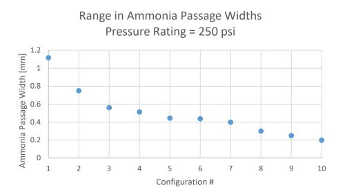
Figure 1. Changes to fabrication parameters result in a range of available ammonia passage widths (0.2-1.2 mm) for the same pressure rating.
