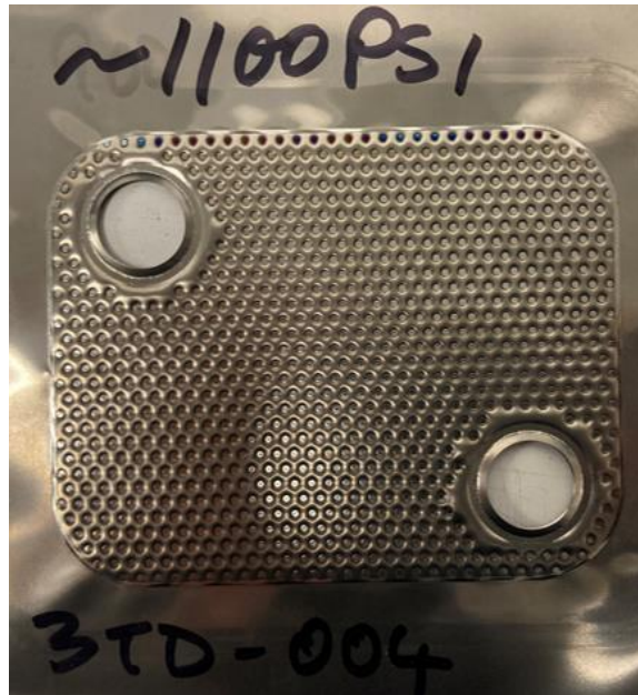
Figure 9. 0.003" short-length plate pressurized to ~1100 psi.
