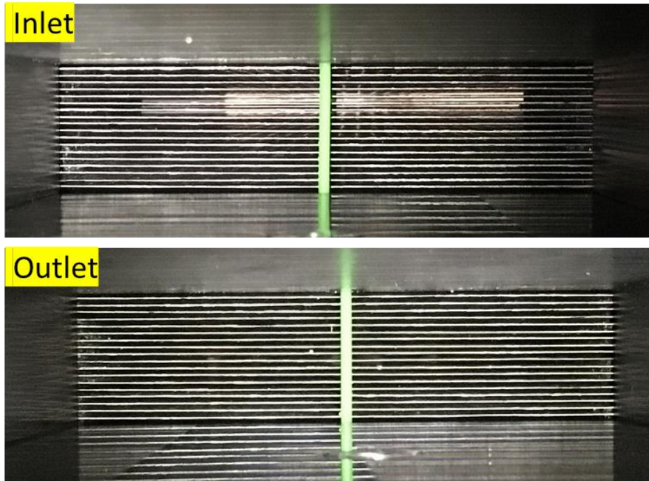
Figure 44. 18-plate stack of TFHX plates. Green comb spacers on the inlet and outlet edges are used to maintain uniform air channels through the test section.
