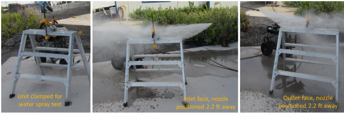
Figure 32. Water spray test setup.
