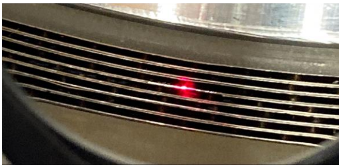
Figure 4. Steps to perform the internal manifold weld include (top) identifying the foil edges and (bottom) welding at the foil edges. The bottom right image shows welds on three adjacent plates.
