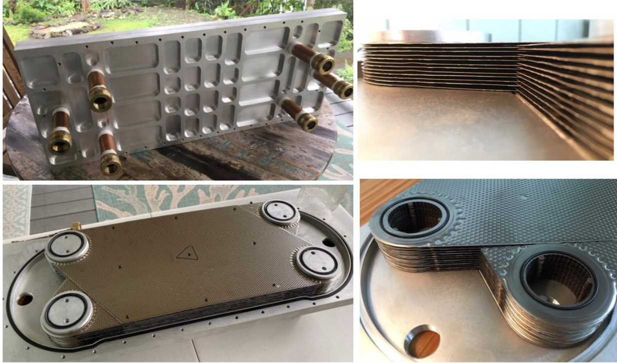
Figure 59. Test HX housing and TFHX plates arranged in the housing.
