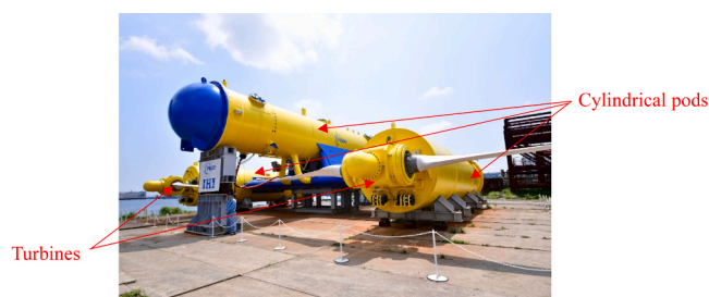
Fig. 2. The kairyu ocean current power generation system. Image reference ( https://t.co/nPNlvwR5Vd ).
