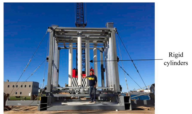
Fig. 12. The Vortex Induced Vibration Aquatic Clean Energy Converter. Image reference (Kim et al., 2021).
