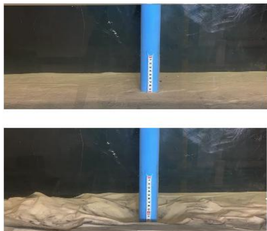
Fig. 10. Scour Testing by AMOG Consulting at the University of Western Australia's O-Tube facility (authors' own). Upper figure is at t=0 , lower figure after several hours of exposure to flow.
