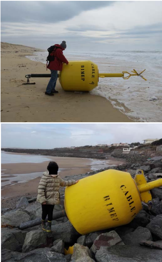
Fig. 5 Connector marker buoys that had broken their moorings found along the French coast
