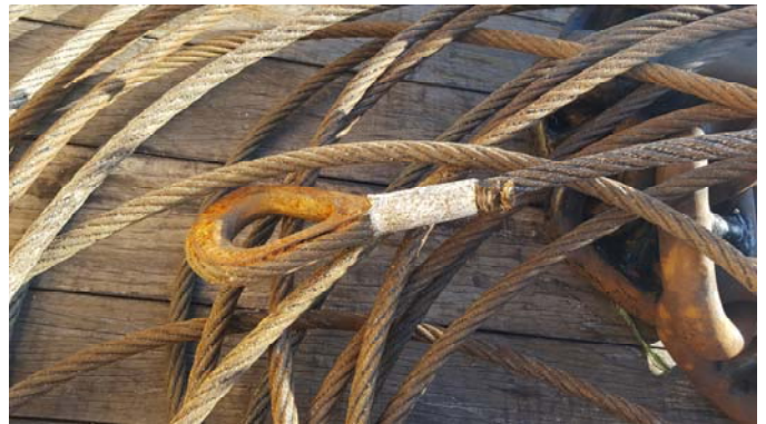
Fig. 6 Aluminium locking sleeve showing corrosion evidence
