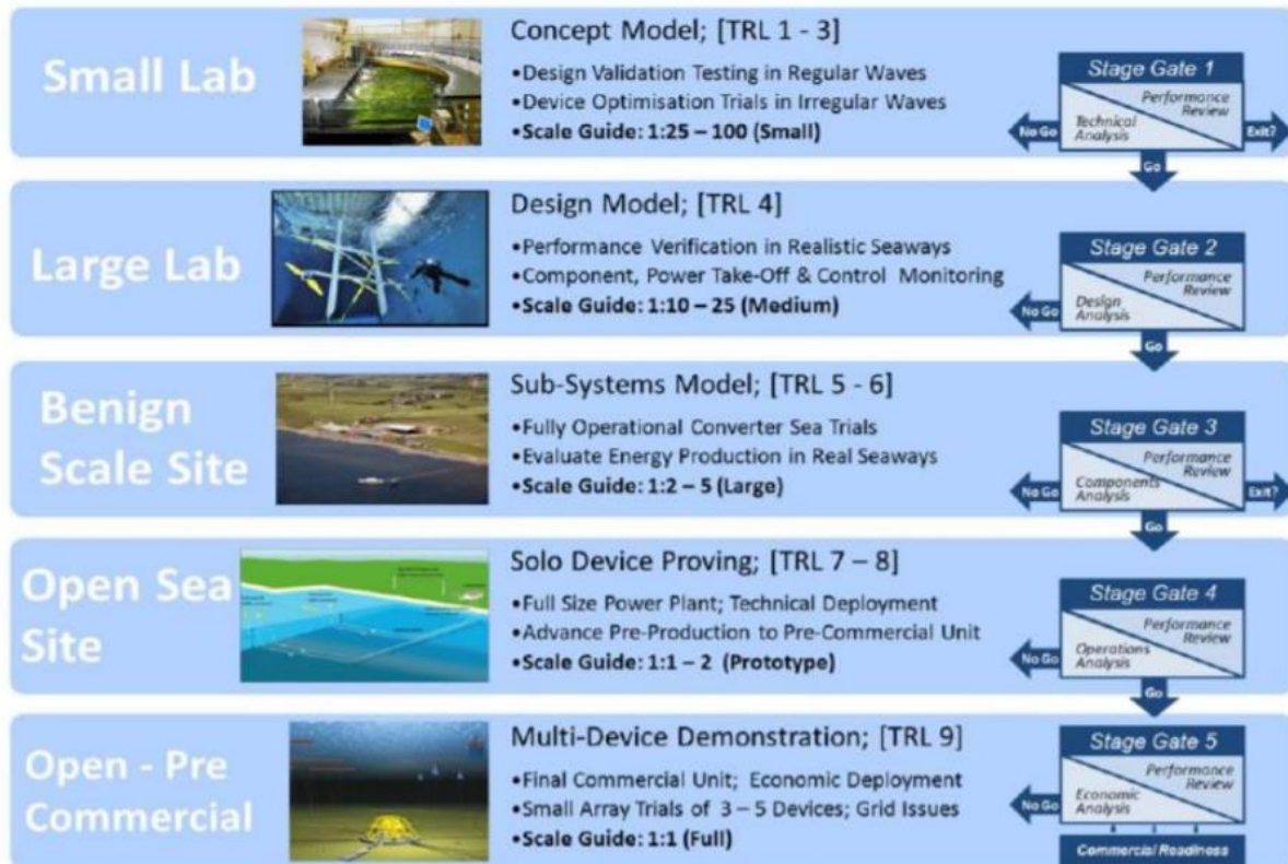
Figure 1-1: TRL description for offshore renewable energy definition
