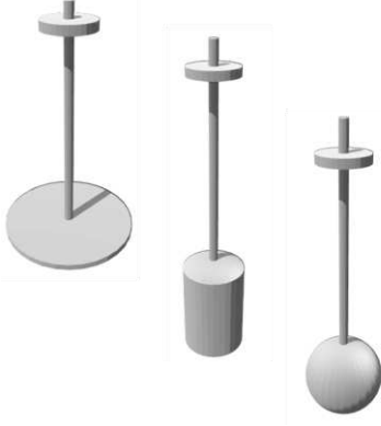
Fig. 2 Configurations of the point absorber using three different submerged body shapes; a plate, a cylinder and a sphere. The top buoy is the same for all three configurations.
