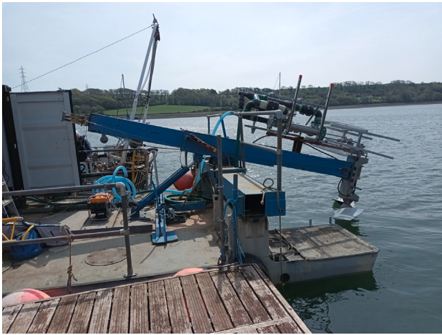
Fig. 7. Full scale turbine and pump assembled to test platform, side view.
