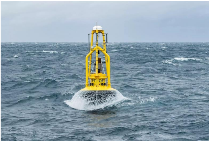
Figure 1: Ocean Power Technologies' PB3 PowerBuoy® WEC [4]
