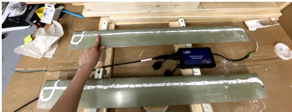
Figure 3: Fiber Optic sensors being embedded in two structural fiberglass composition straight turbine foils
