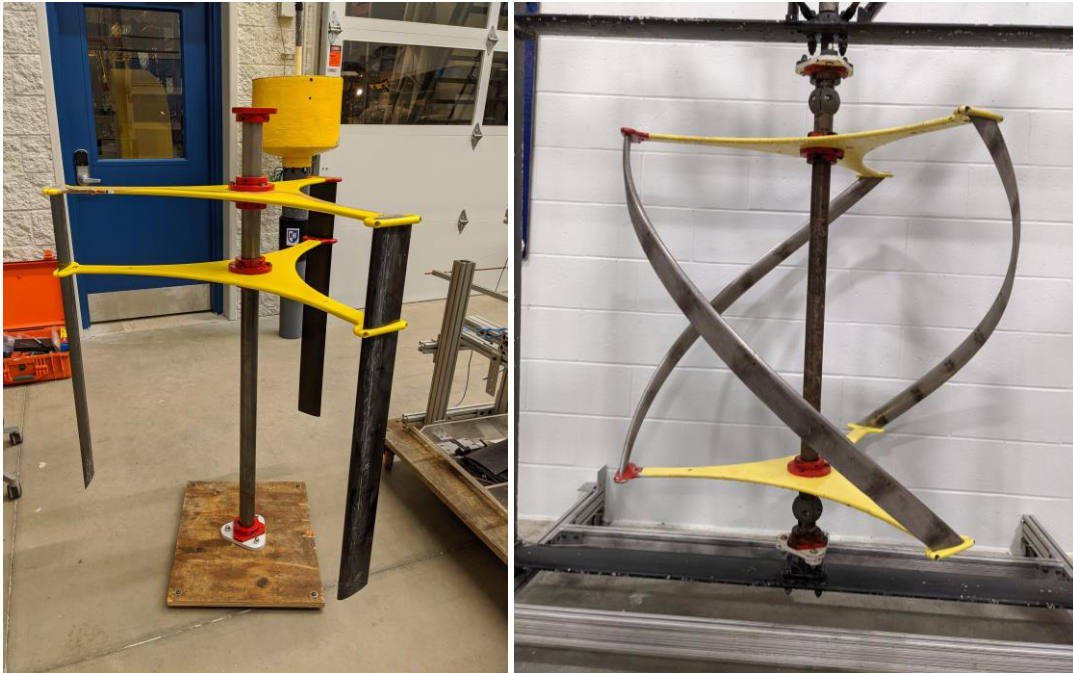
Figure 2: Straight foil turbine and helical foil turbine, showing different positioning of movable strut.
