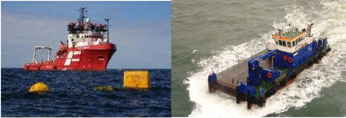
Figure 9-22 Anchor Handling and Multi-Cat Vessels
