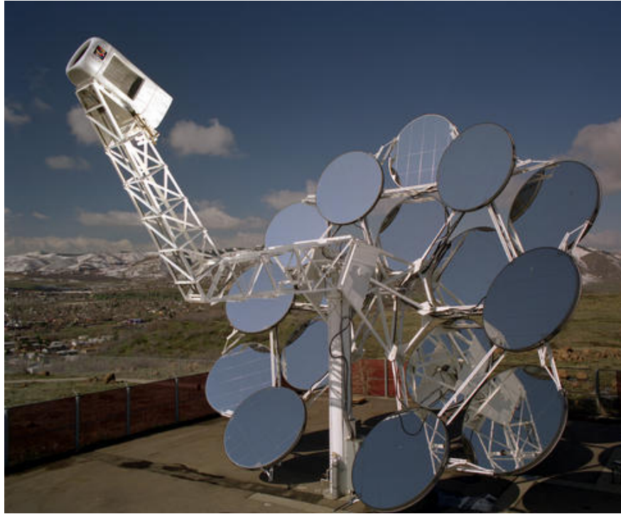
Figure 7-4 25-kW SAIC Dish/Engine System at the DOE Mesa Top Thermal Test Facility. (Source: NREL)
