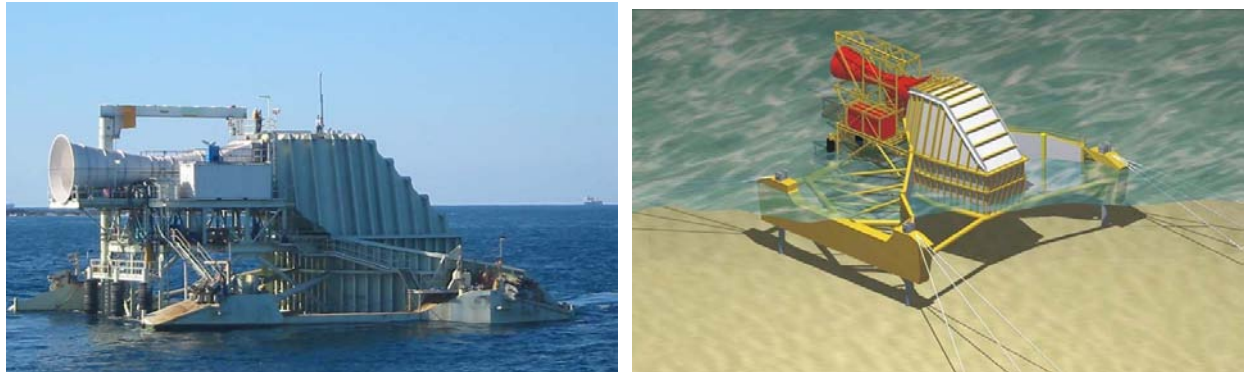
Figure 9-17 Energetech Preproduction Prototype OWC Device Showing Mooring Design
