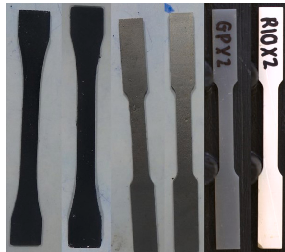
Fig. 1. 3D Printed Dogbone Samples, one of each material. From left to right: Markforged Onyx, Essentium HTN-CF25, Inconel 718, titanium Ti-6Al-4V, Formlabs GreyPro, Formlabs Rigid10k.
