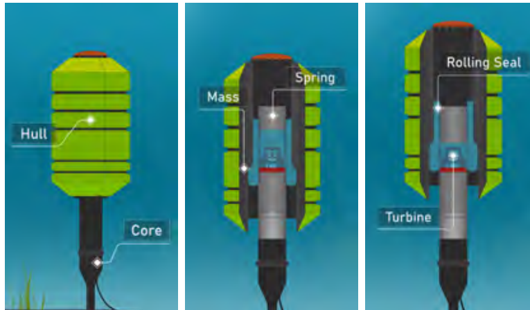
Figure 3.3: Symphony Wave Power’s Symphony internal mechanics [10].
