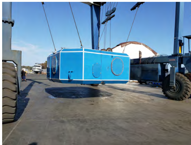
Figure 3.5: CalWave’s xWave pilot out of the water [43].
