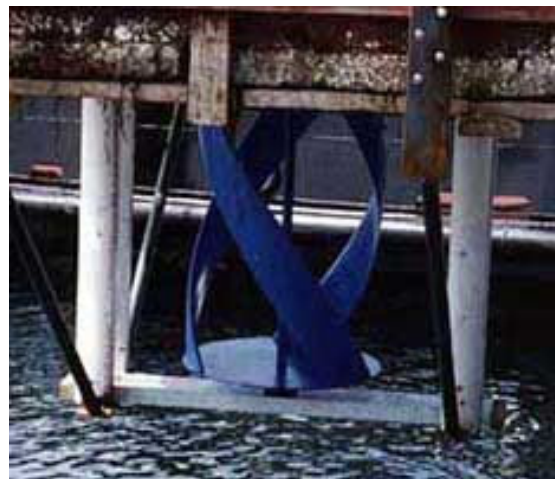
Picture 3: Vertical axis turbine in commissioning
