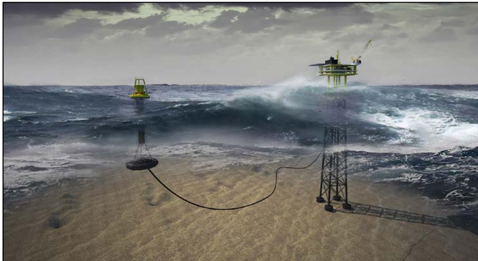
Figure 8: PB40 as a sustainable power source for offshore platform electric power supply and/or diesel generator replacement Concept of operation.
