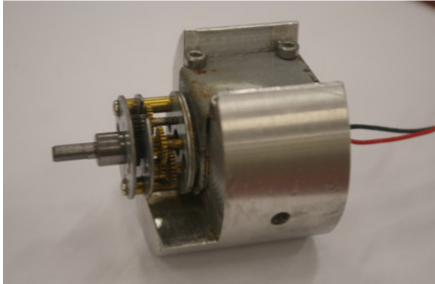
Figure 26. Mounted motor and gearbox.
