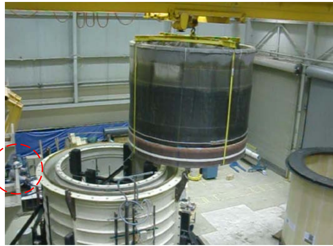
Removing infused and cured workpiece from mold
