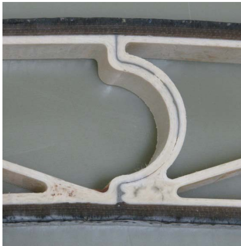
Tongue-in-groove edges of pultrusions
