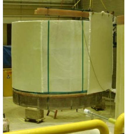
Hanging outer face sheet fabric on test core
