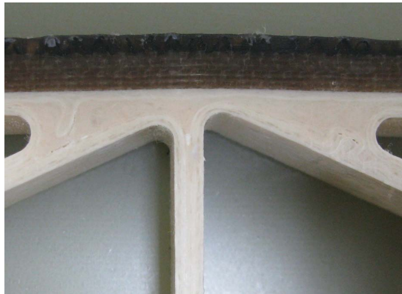
Tongue-in-groove edges of pultrusions
