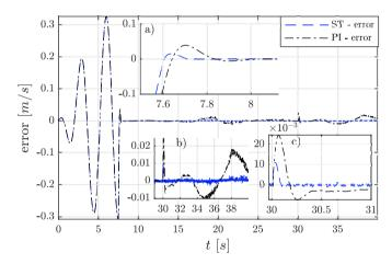
Fig. 7. Error in tracking the reference for both controllers. The error response with the ST controller is shown in dashed blue, while the response with the PI controller is black dash-dot.
