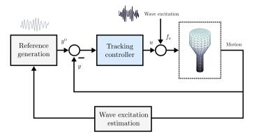
Fig. 1. Typical two-level WEC control architecture.
