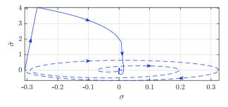
Fig. 5. Super-Twisting convergence in the phase plot  $\sigma$  -  $\dot{\sigma}$ . The dashed lines represent the movement of the system without control and the solid lines the system trajectories under SOSM control.
