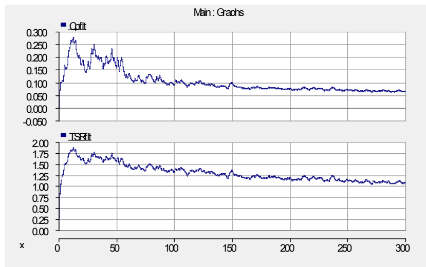
Figure 17. Operating C_p and TSR corresponding to Figure 16
