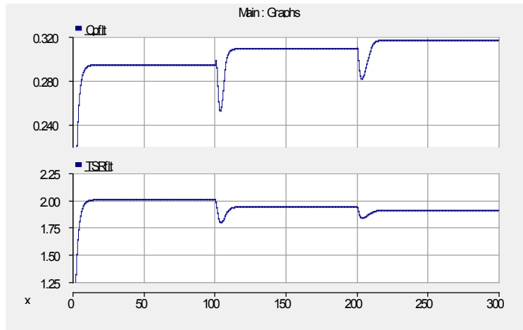
Figure 15. C_p and TSR corresponding to Figure 14
