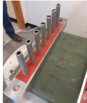
Double-Ended-Insert – metal/composite interconnect
