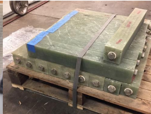
Double-Ended-Insert – metal/composite interconnect
