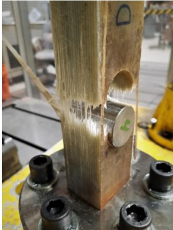
**Figure 10.** A typical through-hole tensile failure of the T-bolt fatigue specimens.
