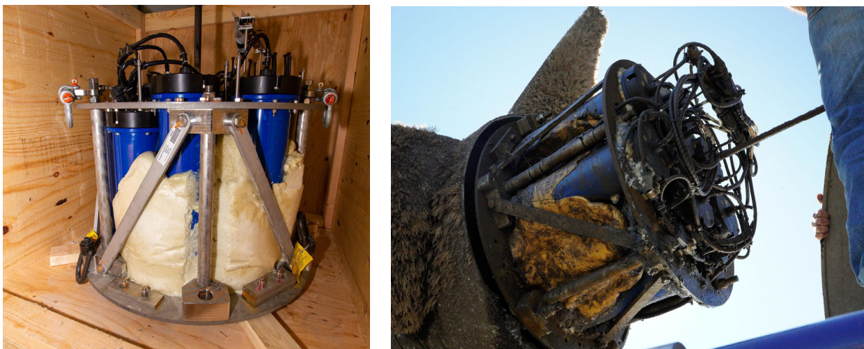
Figure 9. NDAQ with foam fill (left) before deployment and (right) after deployment.
