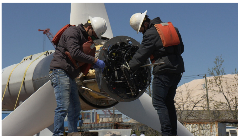
Figure 2. Verdant Power turbine with NREL thermoplastic blades and the NREL data acquisition system (NDAQ).
