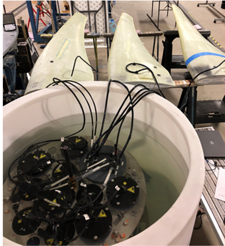
Figure 10. Three thermoplastic blades connected to the NDAQ, and the NDAQ submerged in water.
