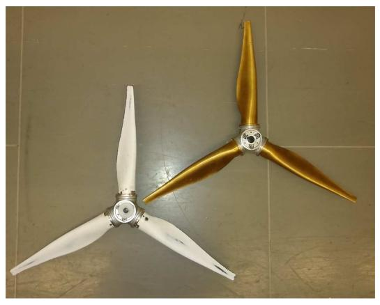
Figure 23: CANOE carbon fibre and SSPA bronze blade, original geometry
