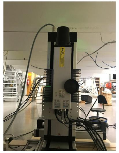
Figure 40 – Solid-state laser and LDV lens.
