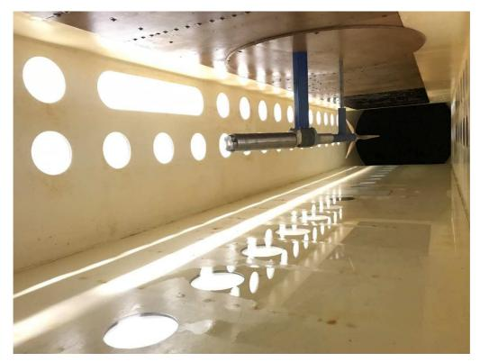
*Figure 43 - Turbine model mounted inside the cavitation tunnel. Measurement windows are visible at the bottom of the test section.*
