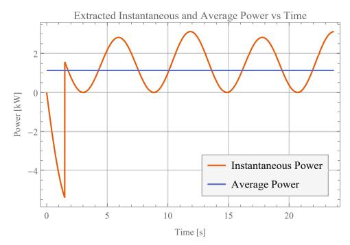
Figure 2.11: Instantaneous and average extracted power from the buoy vs time with initial conditions  $(x0, v0) \approx (0.273, 0)$
