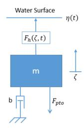
Figure 2.2: Free body diagram of simple dynamic model
