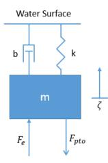
Figure 2.1: Free body diagram of simple dynamic model
