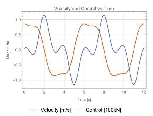
Figure 2.21: Velocity and control force for large (orange) singular arc orbit
