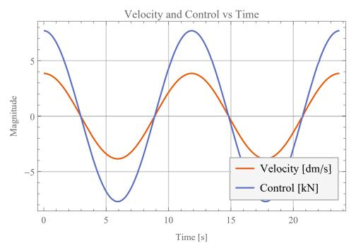
Figure 2.4: Velocity and control force of the buoy vs time. Note that velocity is given in decimeters/second, and control force is given in kilonewtons to make graph scales comparable. The wave field frequency is set at the resonant frequency of the buoy
