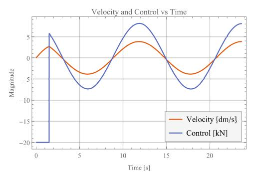
Figure 2.10: Velocity and control force vs time with initial conditions  $(x0, v0) \approx (0.273, 0)$ . Note that velocity is given in decimeters/second, and control force is given in kilonewtons to make graph scales comparable.
