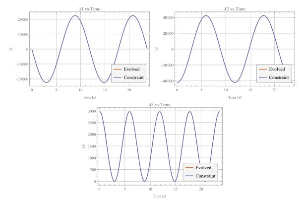
**Figure 2.8:** Co-state numerically integrated (evolved) from the differential equation and calculated from the singular arc constraint
