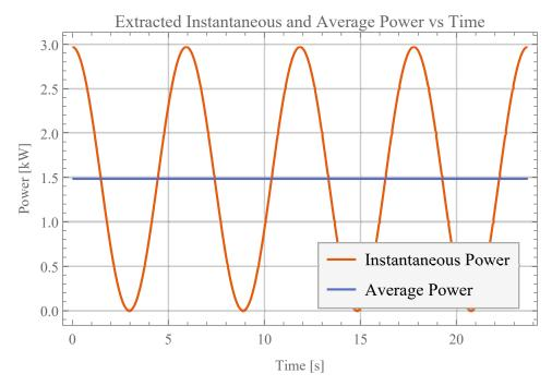
Figure 2.5: Instantaneous and average extracted power from the buoy vs time
