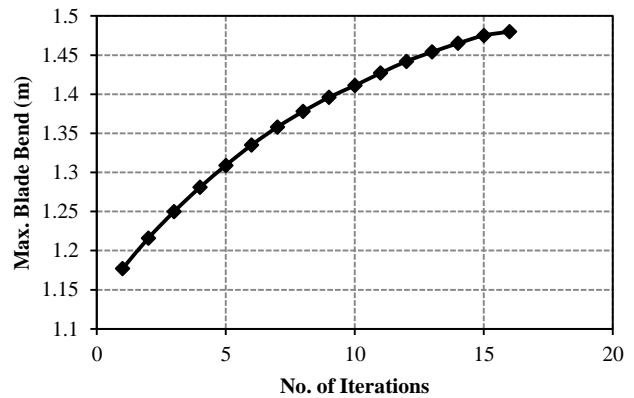
Fig. 10 Number of iterations to convergence of maximum blade bend
