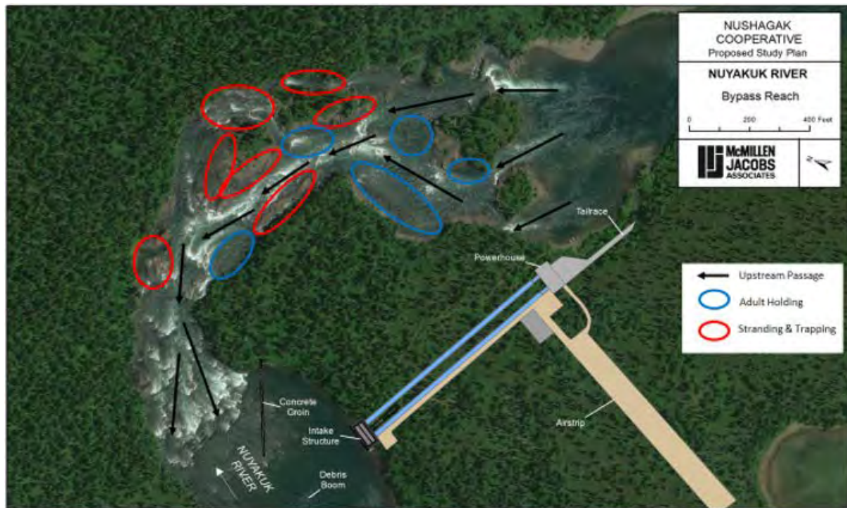
Figure 4-5. Schematic of Nuyakuk Falls Reach showing possible adult upstream migration pathways, adult holding areas, and potential stranding and trapping areas. Photo taken on June 22, 2017; flows approximately 7,200 cfs.
