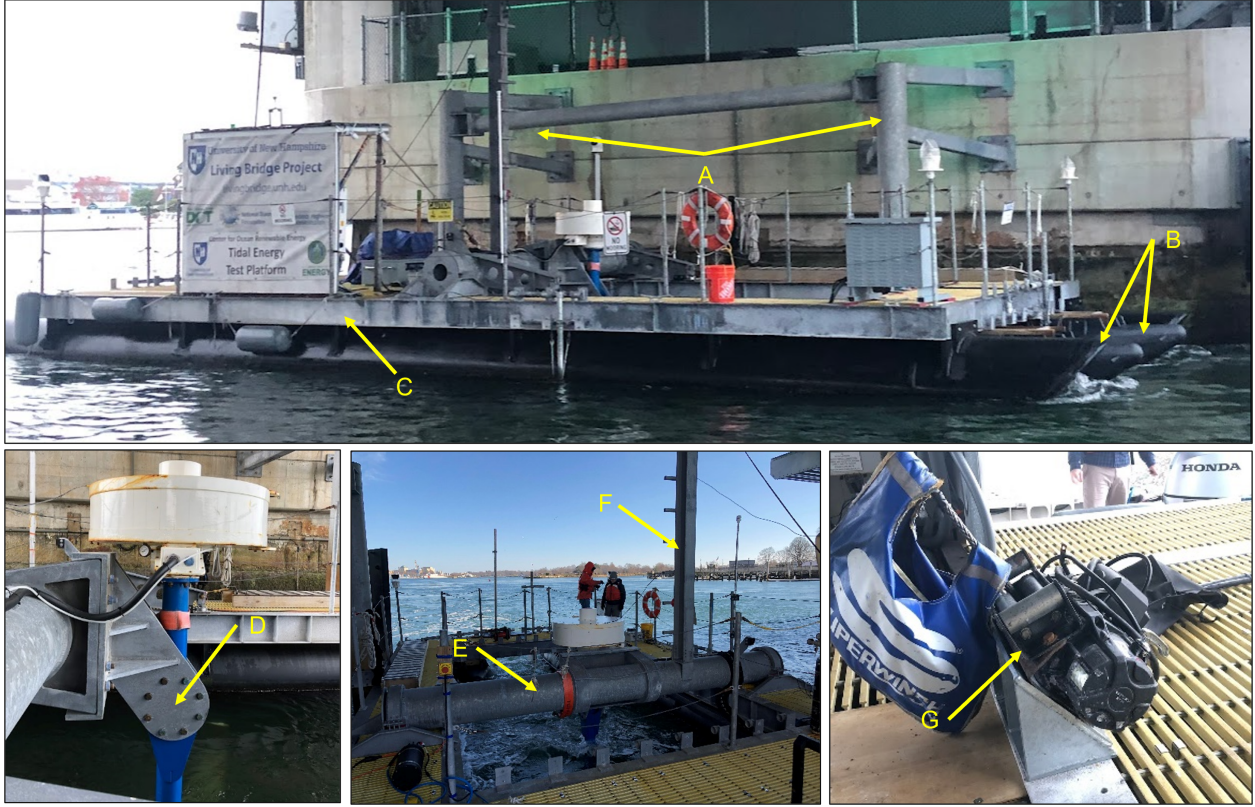
Figure 2.2: An overview of the primary TDP structural and turbine pitching mechanism components. [A] Vertical guide post assembly, [B] HDPE pontoons, [C] TDP steel frame, [D] Adapter bracket, [E] Spanning beam, [F] Strongback, [G] Electric winch.
