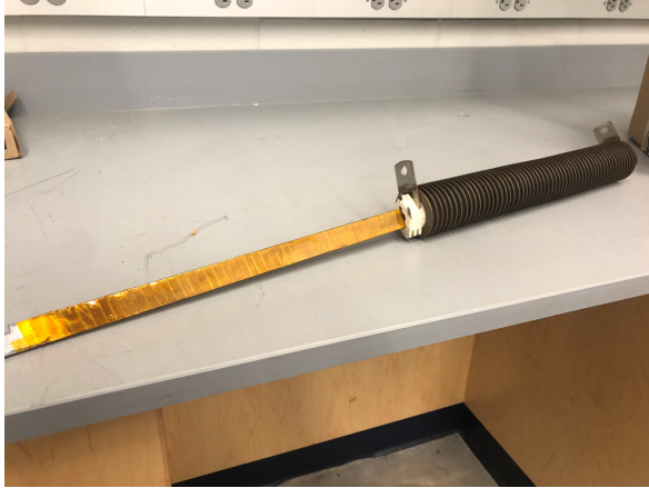
Figure 3.8: [Left] Rebuilt resistor with insulated steel beam. [Right] Bench testing Kapton insulation.
