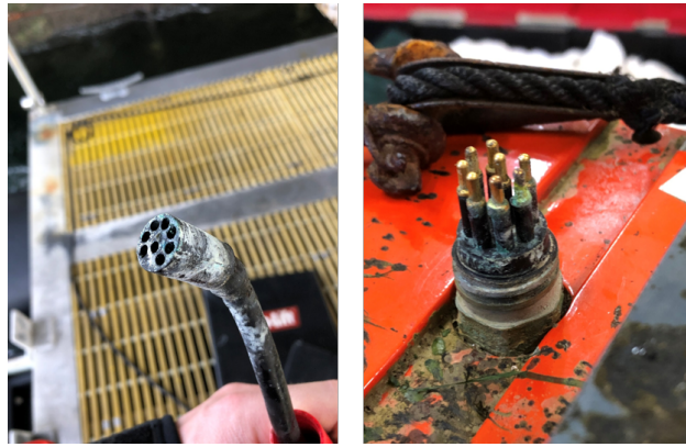
Figure 4.10: Photos indicating the extent of the corrosion present on the bow ADCP data/power cable after the instrument was removed on 12/13/21. [Left] Corrosion evident on SubConn connector. [Right] Corrosion present on bow ADCP bulkhead pin.
