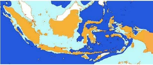
**Figure. 4.** The steepness ( ■ 1,000 m or more depth) of the coastal seafloor of Indonesia as OTEC resources
