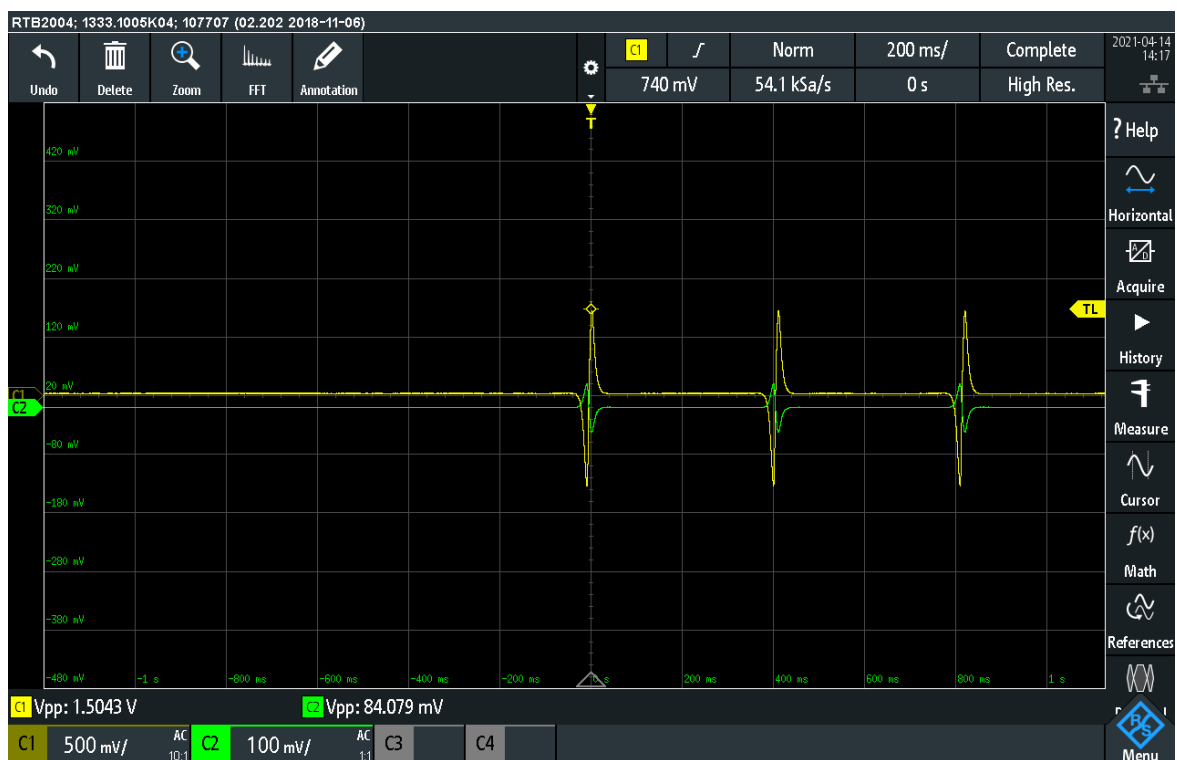
Figure 3.25: Current measurements from the current monitor
