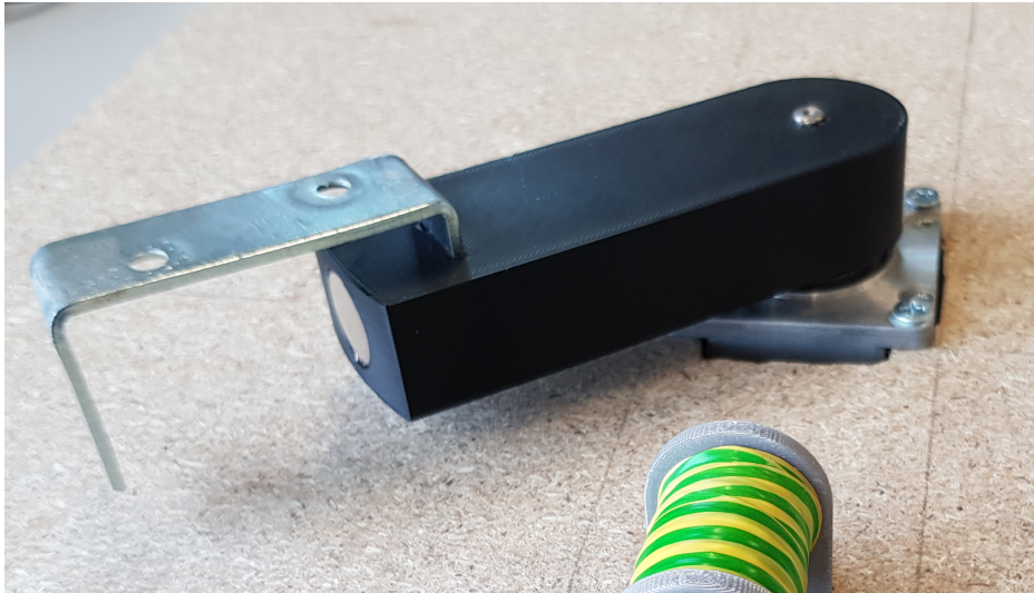
Figure 3.14: Implementation of U-iron in the design
