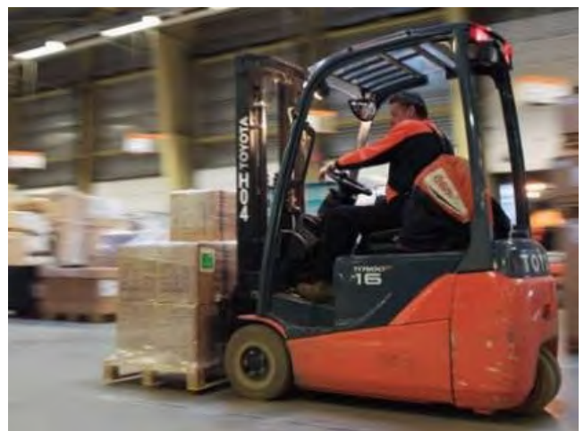
Electric battery forklift. Photo: Toyota Material Handling
