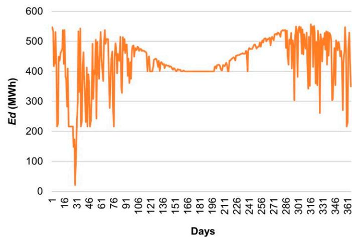
**Figure 8.** Daily dispatched energy,  $E_d$ , from a solar PV farm with 624 MWh battery energy capacity and no tidal energy component. The minimum value of  $E_d$  is 21 MWh.
