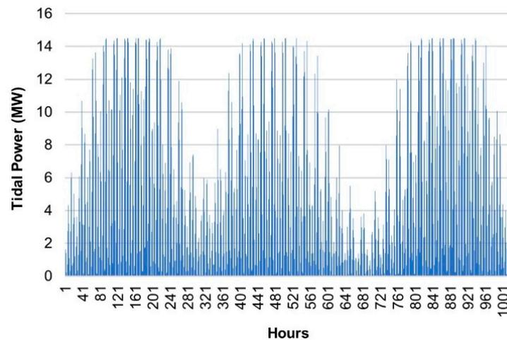
**Figure 15.** Hourly average tidal power generation in Howard Channel using TECs with reduced rated power (uncropped).
