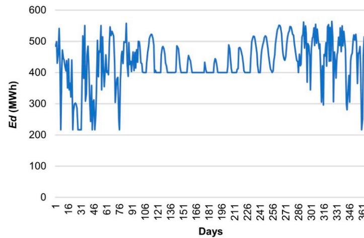
**Figure 6.** Daily dispatched energy,  $E_d$ , from a tidal-solar PV farm with 624 MWh shared energy storage. The minimum value of  $E_d$  is 216 MWh, equal to  $E_{th}$ .
