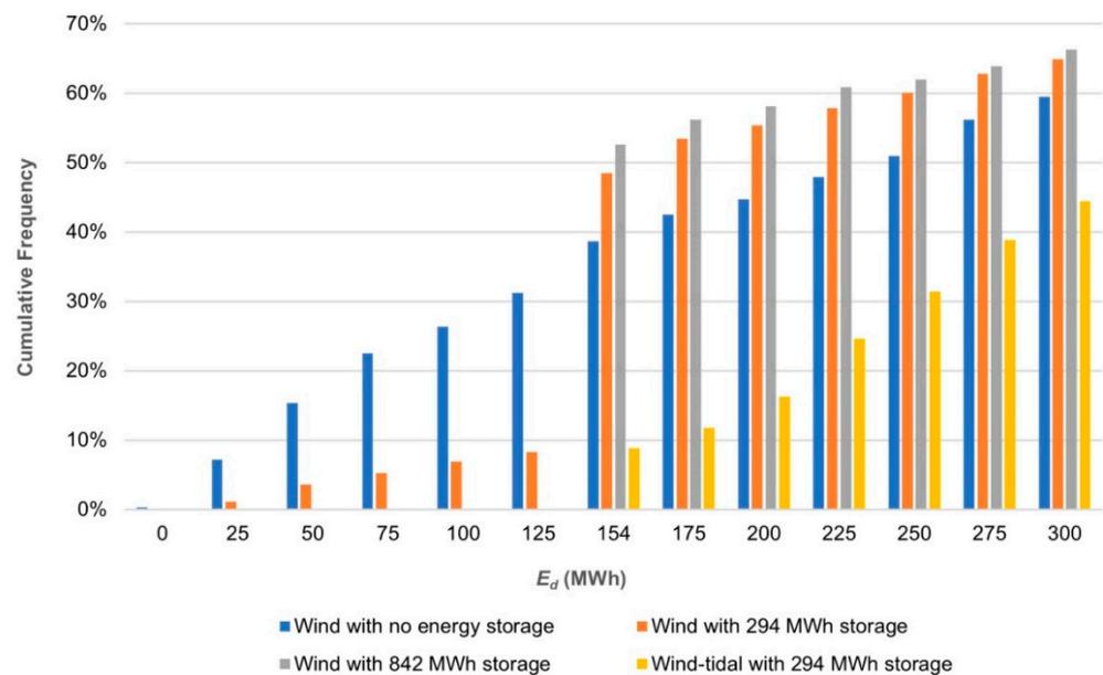
**Figure 13.** Performance comparison of four configurations for a Banks Strait wind farm: (1) wind only, (2) wind with 294 MWh storage, (3) wind with 842 MWh storage, and (4) tidal and wind with 294 MWh storage.  $E_{th}$  is 154 MWh. In configurations 3 and 4,  $E_d$  equals or exceeds  $E_{th}$  (the cumulative frequency of  $E_d$  is zero below  $E_{th}$ ). In configurations 1 and 2,  $E_d$  fails to equal or exceed  $E_{th}$  for 31% and 8% of the time, respectively.
