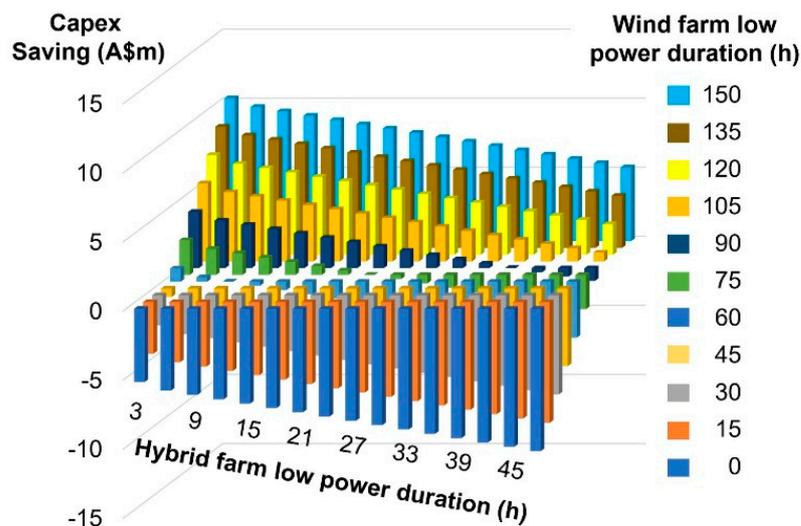
**Figure 11.** The CAPEX saving dependence on low power duration in a tidal-offshore wind farm and in a stand-alone offshore wind farm. (Equation (5) with:  $P = 1$  MW,  $P_{tidal} = 0.5 \times P$ ,  $P_{th} = 0.3$  MW,  $CF_{tidal} = 0.18$ ,  $CF_{wind} = 0.45$ ).
