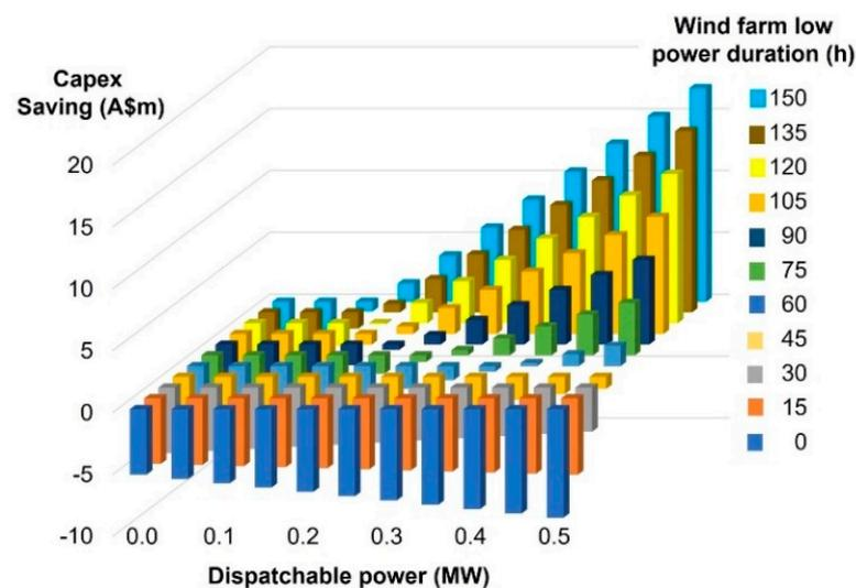
**Figure 9.** The CAPEX saving dependence on the dispatchable power threshold and low power duration in a standalone offshore wind farm, (Equation (5) with:  $P = 1 \text{ MW}$ ,  $P_{tidal} = 0.5 \times P$ ,  $\tau_{tidal} = 20 \text{ h}$ ,  $CF_{tidal} = 0.18$ ,  $CF_{wind} = 0.45$ ).
