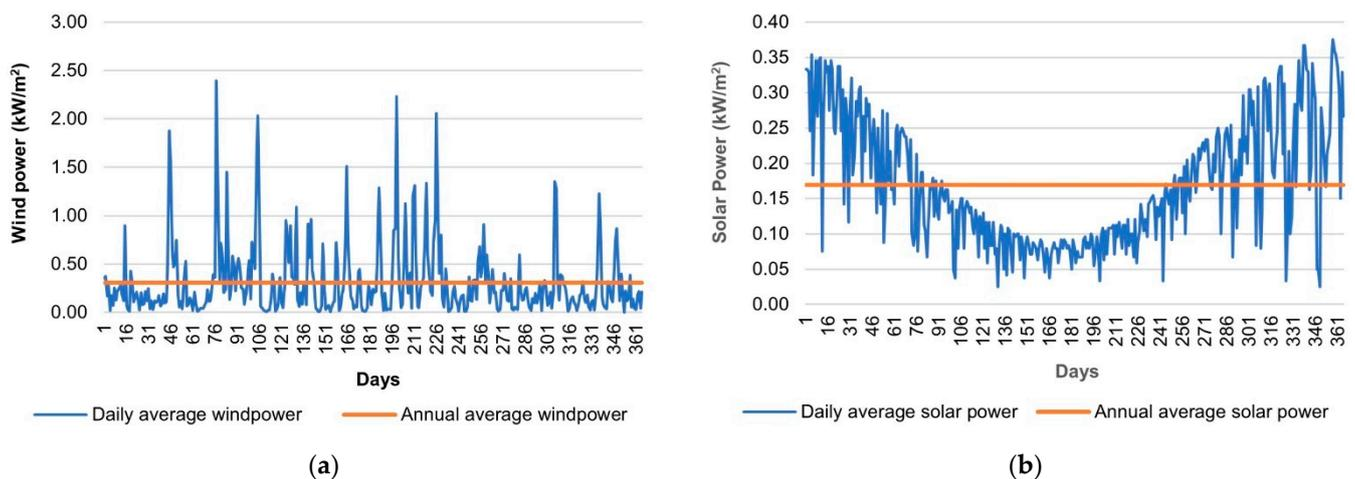
**Figure 4.** Swan Island Banks Strait: (a) Wind power intermittency; (b) Solar power intermittency and variability.
