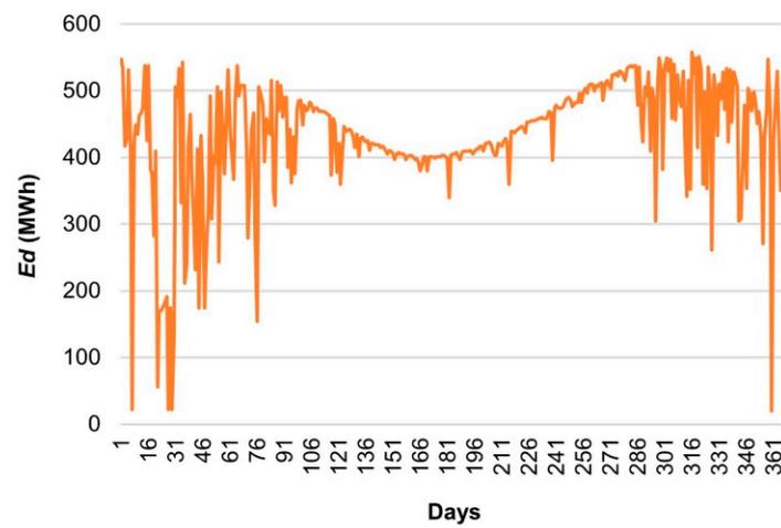
**Figure 5.** Daily dispatched energy,  $E_d$ , from a solar PV farm with no energy storage and no tidal energy component. The minimum value of  $E_d$  is 21 MWh.
