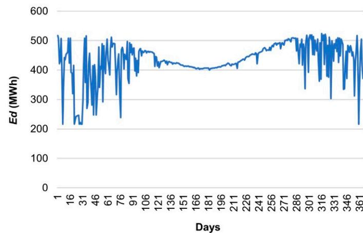
**Figure 7.** Daily dispatched energy,  $E_d$ , from a tidal-solar PV farm with a 624 MWh shared battery energy capacity. The chart averages 30 tests with phase differences between the solar and tidal energy minima ranging from 0 to 29 days. The improvement in  $E_d$  exceeds or equals  $E_{th}$ .
