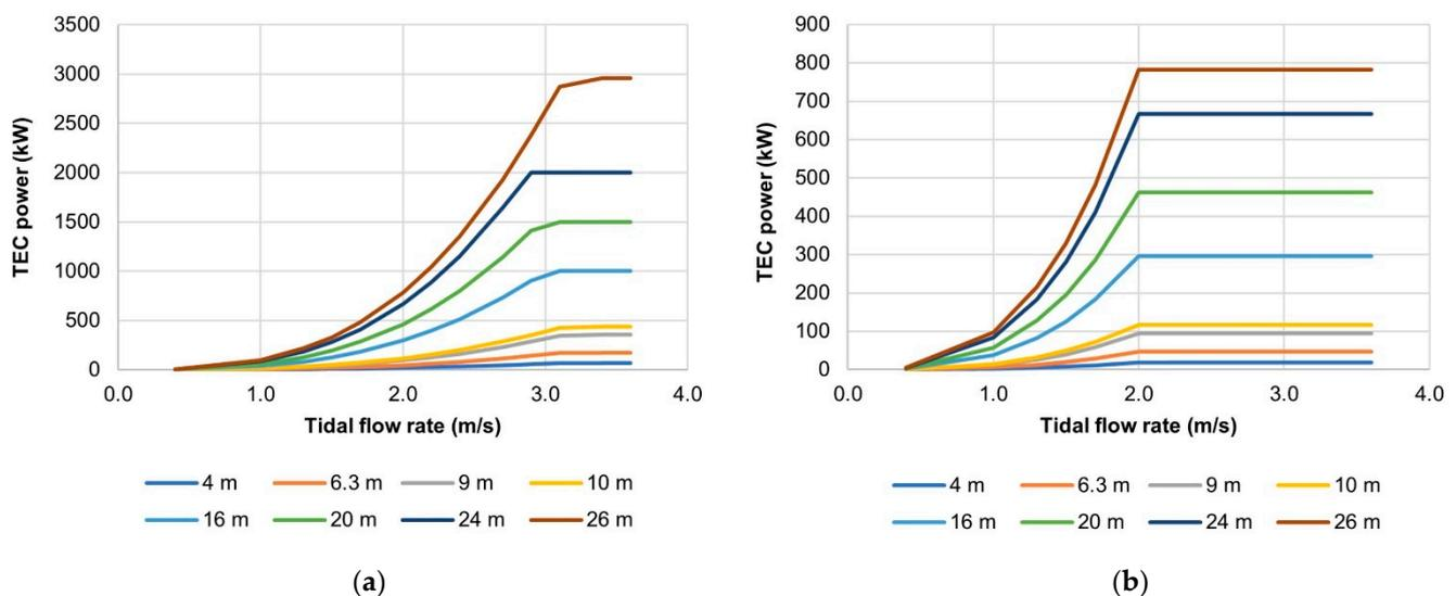
**Figure 2.** Generic power curves for TEC rotor diameters ranging from 4 m to 26 m: (a) based on commercially available TECs; (b) matched with the Australian tidal energy resource [6]. Copyright UTAS 2020. Adapted with permission.
