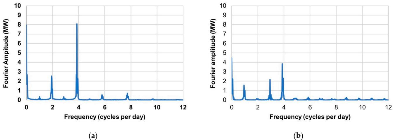
**Figure 3.** FFT spectra for tidal farm hourly average electrical power samples from: (a) Banks Strait; (b) Clarence Strait. The half cycle of the period corresponding to the line at 3.9 cpd determines the low tidal power period (3.1 h) requiring battery support. The folding frequency was 12 cycles per day and the sample size was 1024 including three zero pads.
