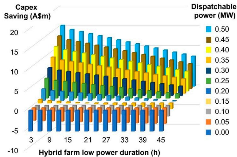
**Figure 10.** The CAPEX saving dependence on dispatchable power and low power duration in a tidal-offshore wind farm. (Equation (5) with:  $P = 1$  MW,  $P_{tidal} = 0.5 \times P$ ,  $\tau_{wind} = 119$  h,  $CF_{tidal} = 0.18$ ,  $CF_{wind} = 0.45$ ).
