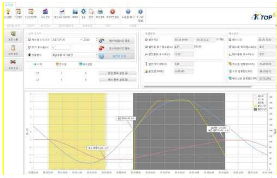
Fig. 22. K-TOP Program Screen for Calculating Power Generation of Shihwa Tidal Power Plant.
