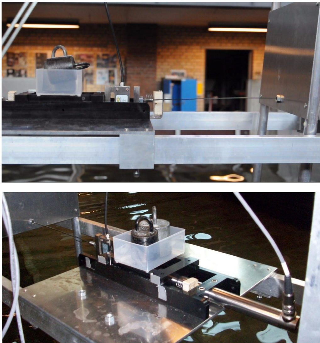
Figure 4 and 5: The PTO system, including the force transducer, the load setting by weights and the LVDT.
