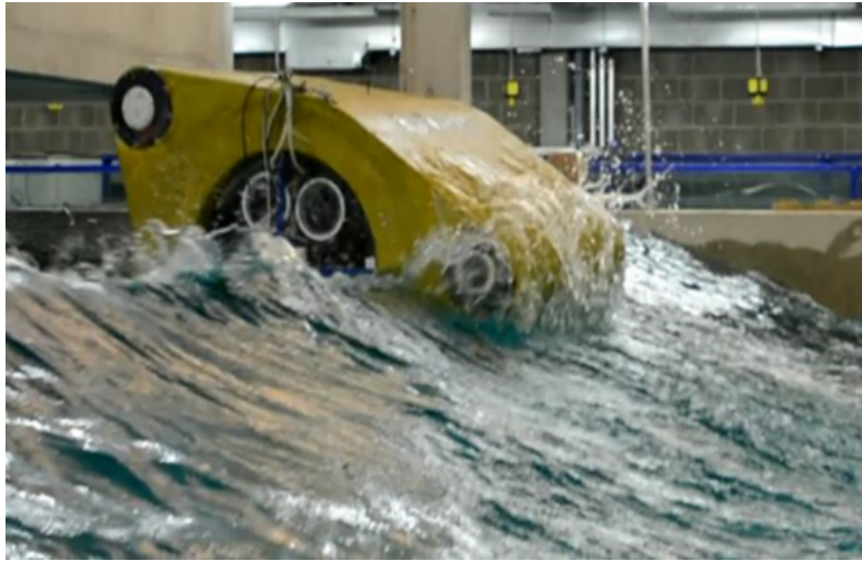
Figure 2. Physical scale model testing of the Pitching WEC.
