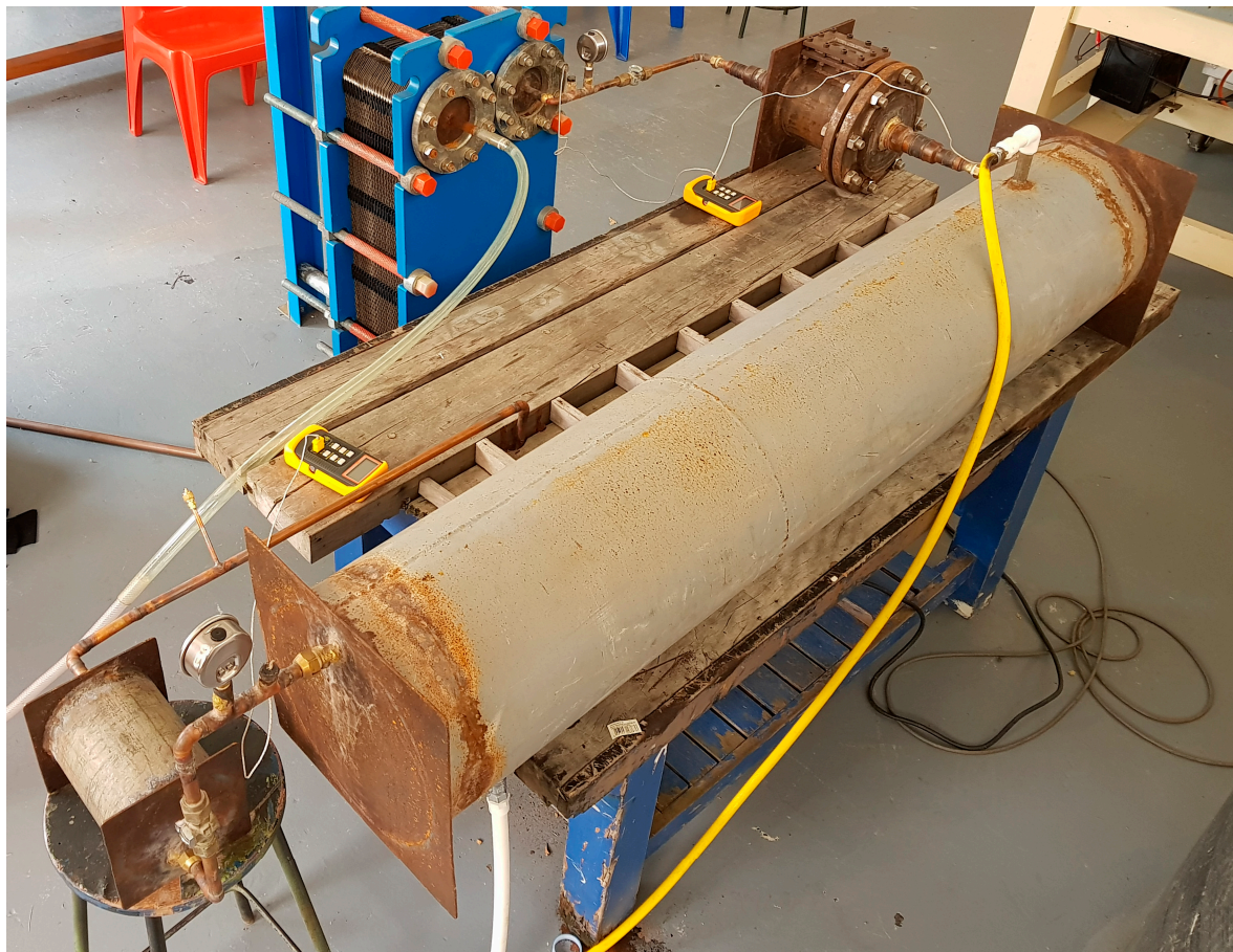
Figure 7. A closer view of the shell-and-tube heat exchanger that was used as a condenser.
