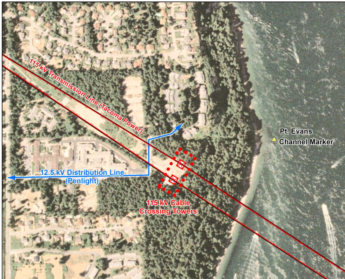
Figure 2.14 – Interconnection infrastructure near Point Evans, Tacoma Narrows
