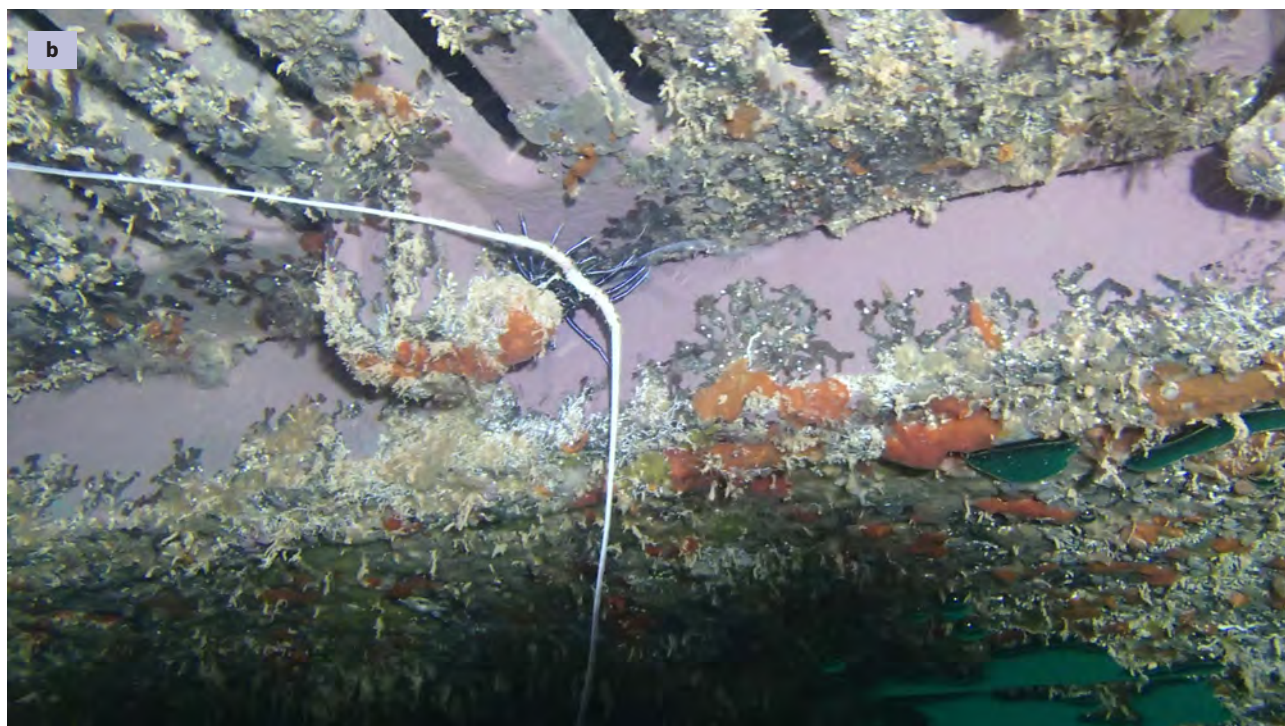
Figure 2.5 a) Typical sea chest arrangement showing sea chest location and fouling. Source: David Smith; b) Internal sea chest fouling. Source: Ashley Coutts (Biofouling Solutions Ltd).
