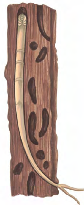
Figure 2.2 Illustration of shipworm burrowing into timber. Source: Ekaterina Gerasimchuk/Shutterstock.
