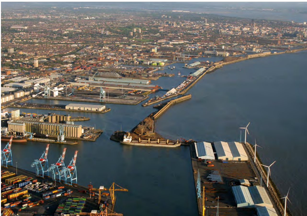
Figure 4.5 Typical wet dock port arrangement.
