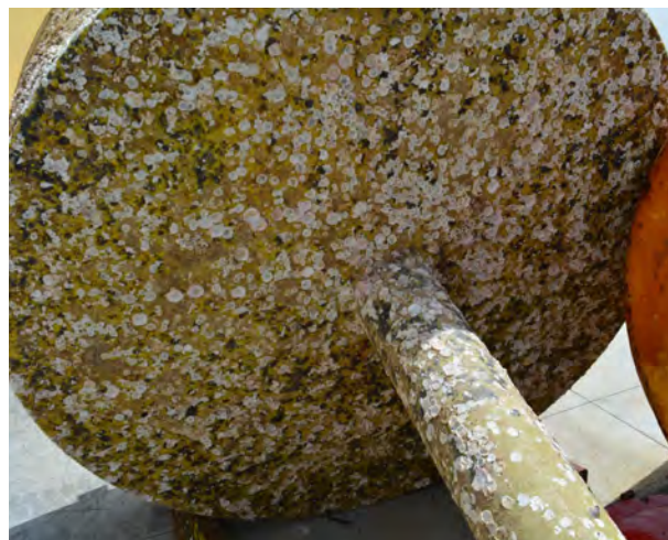
Figure 1.12 Monitoring buoy after being cleaned, showing remains of barnacles not removed by standard cleaning practices.
