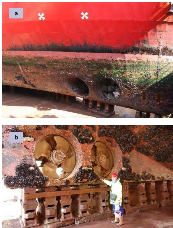
Figure A5 Niche areas – Manoeuvring (a) bow and (b) stern thrusters. Source: David Smith.
