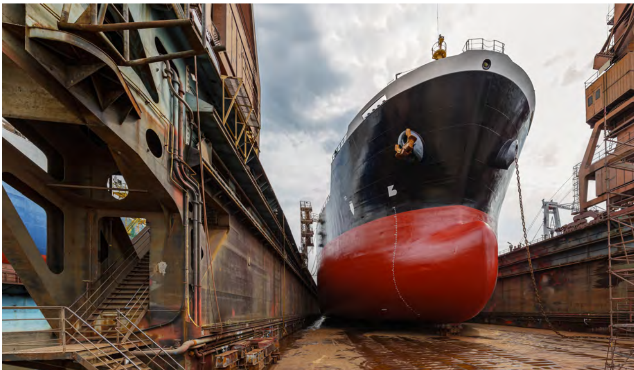
Figure 4.2 Large tanker hull designed for maximum cargo volume at slower speed have greater operating draft and considerably larger WSA when fully loaded.
