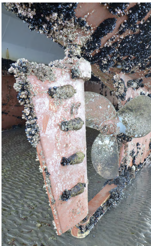
Figure 1.2 Macrofouling consisting of barnacles and mussels.
