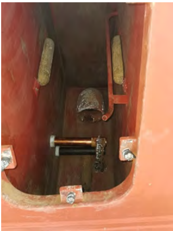
Figure A15 Typical copper anode arrangement in a sea chest.
