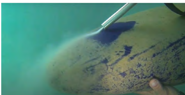
Figure 4.24 Diver-controlled, in-water cleaning devices: a. A scuba diver removing biofouling (including the invasive ascidian Ciona robusta and the Mediterranean mussel Mytilus galloprovincialis ) from the hull of a recreational boat, using a metal scraper and a net to capture the material. Source: A. Plos; b. Remora. Source: www.remoramarine.com ; and c. CavitCleaner with Tornado 2. Source: www.cavitcleaner.com .
