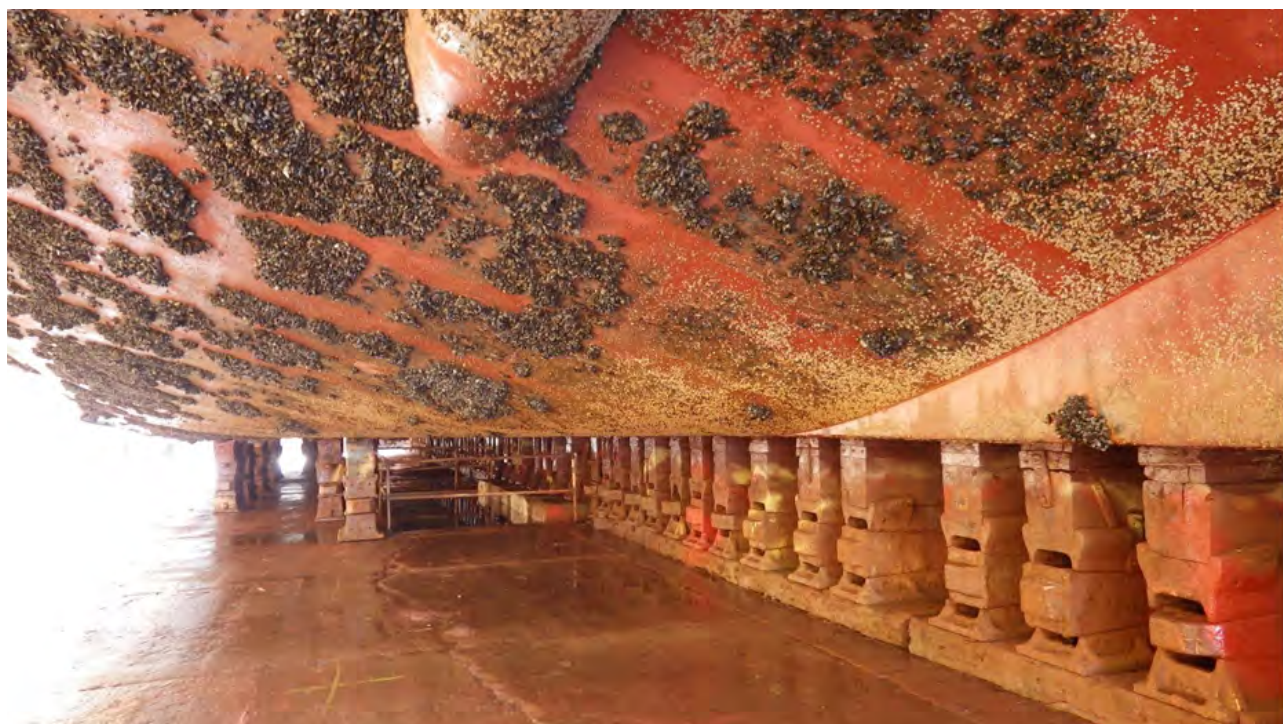
Figure 4.3 Underside of a ship's hull showing extensive fouling.
