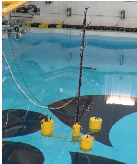
Hybrid model test with multi-propeller actuators at UI Hydraulics Wave Basin Facility.
