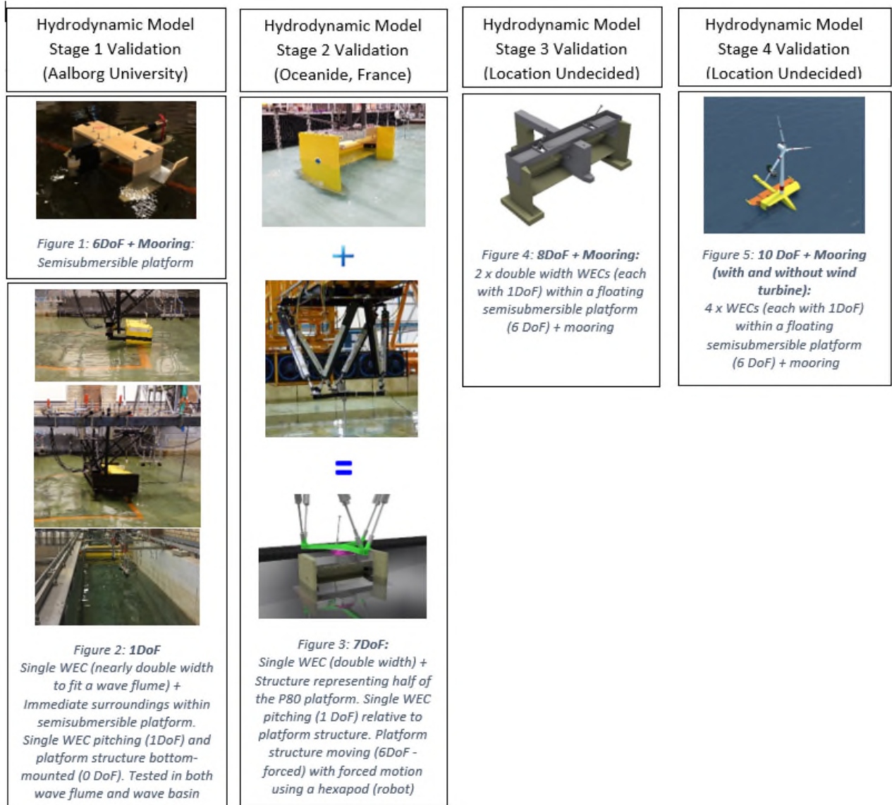
Figure 1: Plan for FPP Hydrodynamic Model Development and Validation
