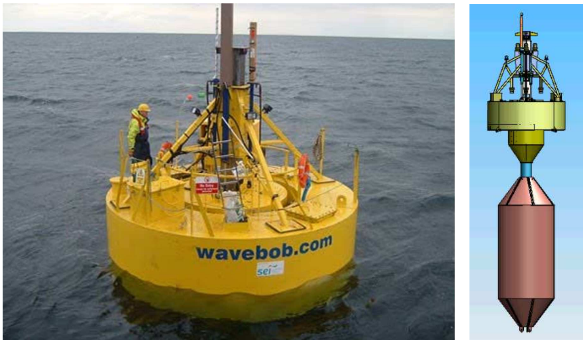
Figure 7.11: WaveBob 1:4 device tests (left) and full-scaled design (right).
