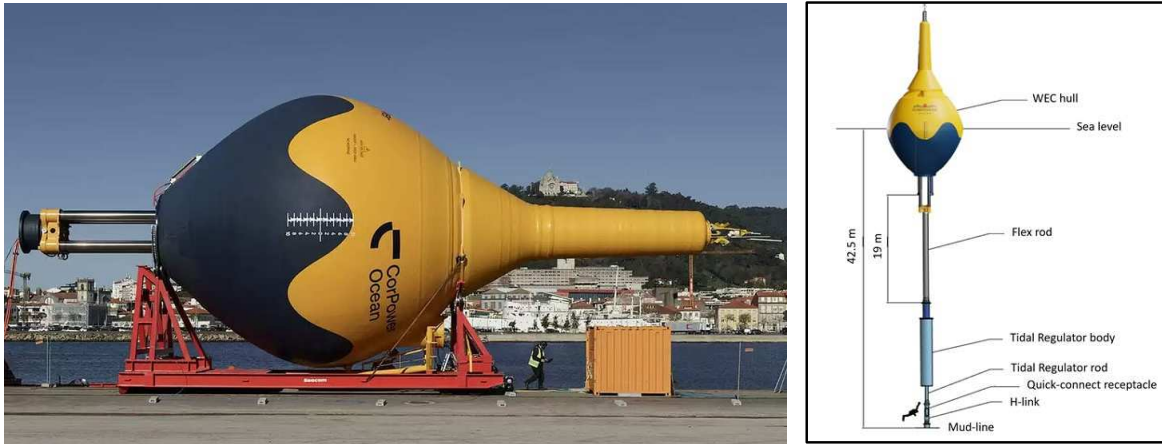
Figure 7.13: CorPower C4 hull (left) and schematic (right).
