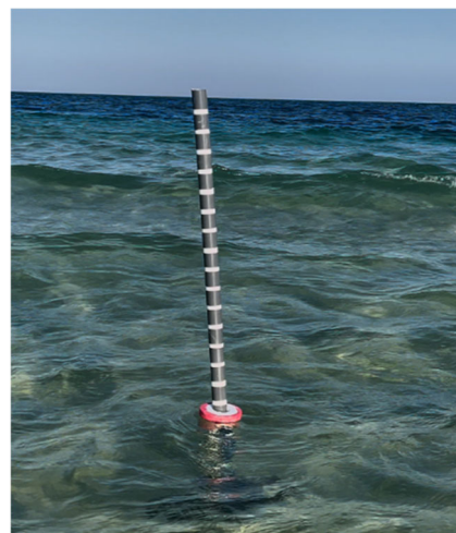
Figure 3. Calibrated rod and small buoy used for on-site wave motion and height measurements.
