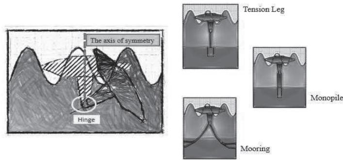
Fig. 2 Absorbing energy mechanism and support structures
