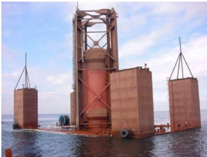
Fig. 5. Archimedes Wave Swing pilot plant [15].
