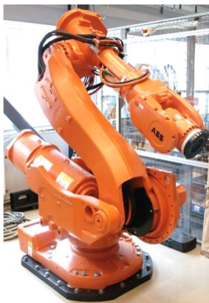
Figure 5. 6-DOF industrial robot manipulator used as wave-maker during the experiments.
